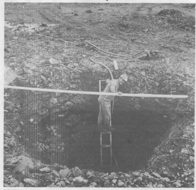
PAT DROZDA (6258) stands on a ladder in a 3-metre-deep, 4-metre-diam. hole formed during an explosive experiment in Kentucky's Straight Creek coal mine. The blast, one of a series last summer, is part of Sandia's program to verify mathematical models that can be used to plan cast-blasting operations.
